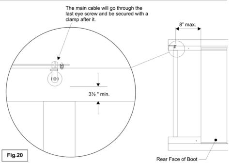
side of the drum and tighten a clamp onto it so as to stop it from going back. Put the main lift cable under tension with the drive, making sure not to over tighten it, i.e. pulling out the last eye screw. The cable should be taught.
