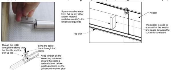
**25.** It is important at the end in which the secondary cable installation begins is secured by an extra 3 1/2" nail into the building structure (in two hookups). This will keep the retainer pipe from shifting sideways during installation. Complete all cable hookups. Finally remove the clamp after the last eye screw that is holding the tension on the main cable.
