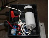
46. Connect red wire from slack detector to black power wire. Connect other black wire to motor side.
