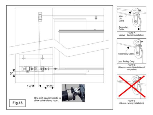
20. Hooking up the main cable: At the drive end, ensure the cable is through the corner drop pulley and run down to the drive. Cut the cables so that it hangs 15" past the drum. Run the cable down behind the drum then wrap all around the drum. Now pass the tail end through the hole in the end plate of the curtain
