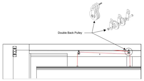
**17.** Install the typical or standard pulleys along the opening. (The typical/ standard pulley wheel must be spaced at a greater distance than the curtain opening.)
