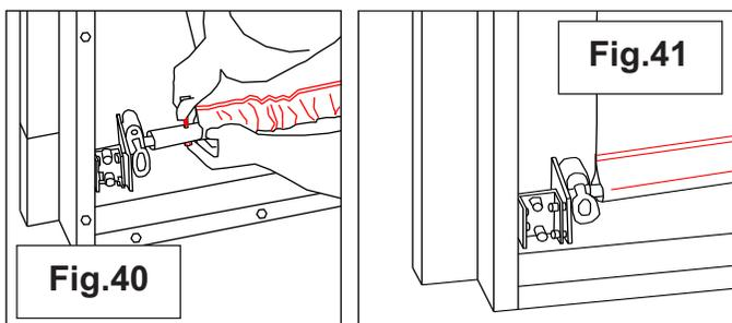
41. The gearbox is now installed and should look as shown:
